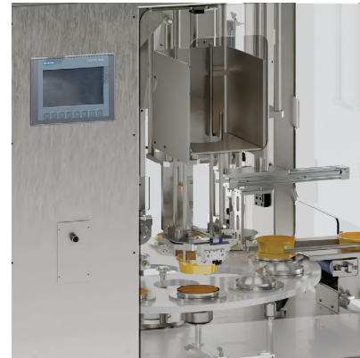
Operator HMI touch screen
